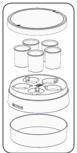
**H5D-F01**: Borosilicate-glass-bottom 0.16 mm; wall: polystyrene; 1 pkg. / 5 pcs. With carrier element and HiCult as protective dish
